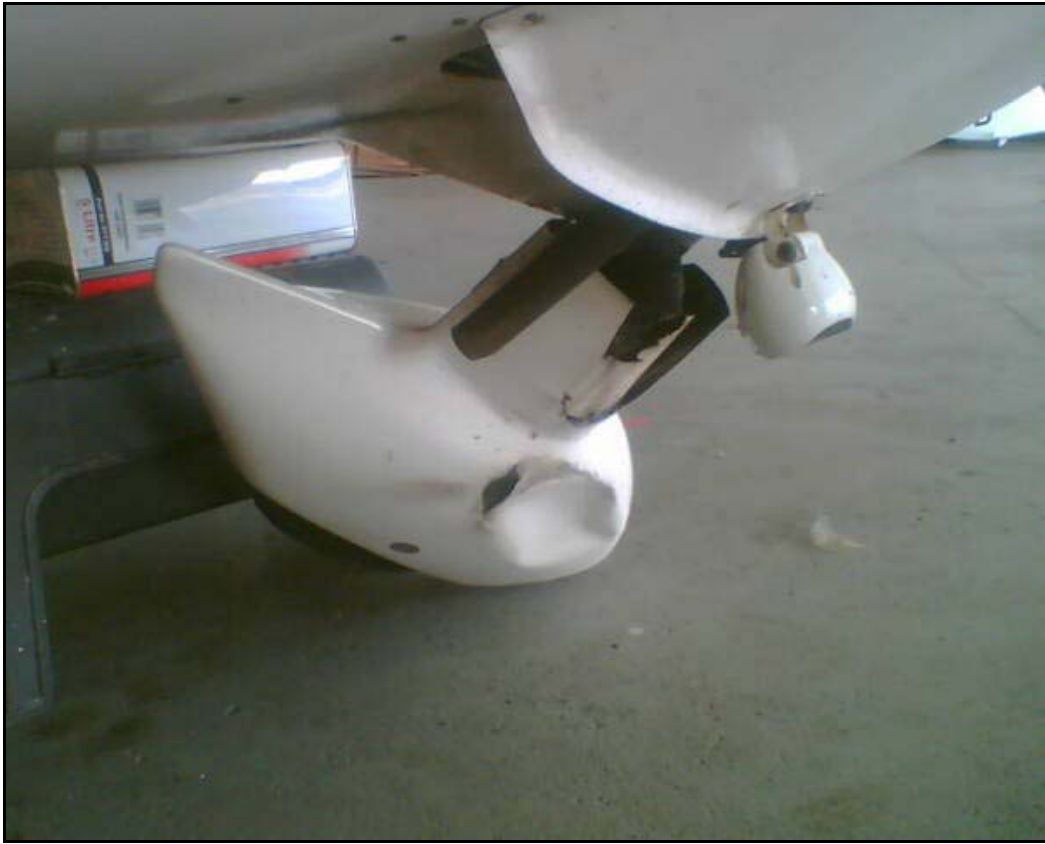
Photo No.1: The bent nose undercarriage following the incident.
