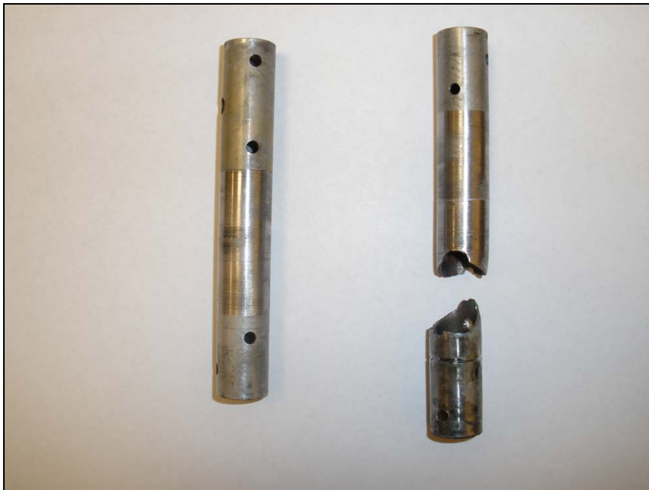
Photo No. 1: The intact LH pillar and the failed RH pillar.
