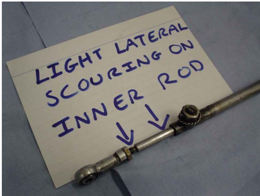
Photo from engine contractor showing other end of linkage with score marks on inner rod.
