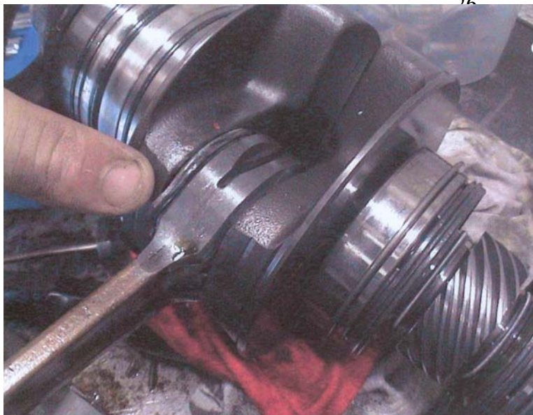
The thumb points to the engine connecting rod and associated big-end bearing which failed in service on G-CBFT.
