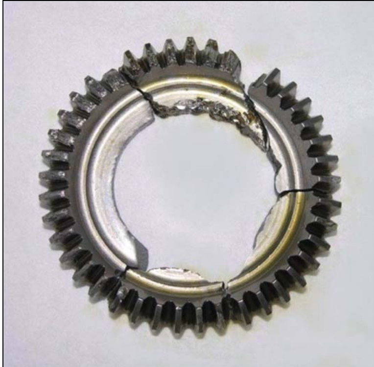
Fig. 2 Bevel gear fragments
